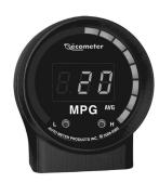
You can select the target fuel economy (MPG) for your vehicle by pressing and holding the right (data input) button while in instantaneous MPG mode. The display will show a target MPG which will increase from 5 to 50 in increments of 5 MPG. Continue to press the right button until your target MPG is displayed, then release. This target MPG will then translate to an ecograph with the top green LED illuminated.
