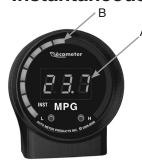
Under this mode the digital display (A) will show the real time fuel economy (miles per gallon) that your vehicle is currently achieving. The ecograph (B) will show you how efficiently you are utilizing the fuel in your vehicle. The more green bars, the more efficient.
