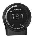
Pushing the right button while in MPH mode will display the maximum MPH (speed) the vehicle has reached. While displaying the maximum value, the MPH indicator will flash. To clear the maximum MPH value, push the right button a second time (within 5 seconds of entering maximum mode).
