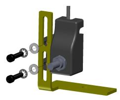
Find location for the sender on the transmission. Either in front of the shifter lever (1) or behind the shifter lever (2)
