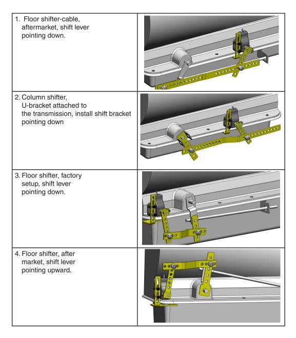
By making simple modifications to the shift bracket and the linkage, the sender can be adapted to fit to many transmission configurations. The linkage comes with a preset offset. Adjustments can be made by simply in creasing or decreasing the pre-existing bends.
