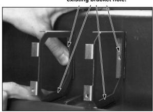
8. 2%" gauges require mounting brackets to hold them in place (see gauge instructions for mounting).
