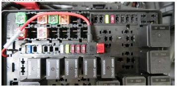
99. Feed the fuse tap wire on the Water Pump harness through the opening of the fuse box as shown. Using crimpers, connect the fuse tap wire to the butt connector installed on the fuse tap.
