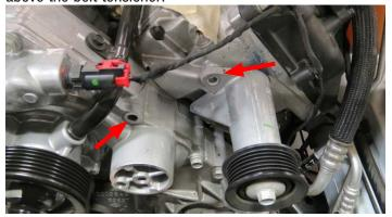
50. Using the short spacer and the bolts from Bag #2, loosely mount the idler bracket to the two bolt hole locations from the previous step. Using the long spacer and M6  $\times$  110mm bolt from Bag #2, secure the bracket to the third bolt location; the provision on the cylinder head above the idler pulley bolt removed from Step 49. Torque all bolts to 21 ft/lbs.
