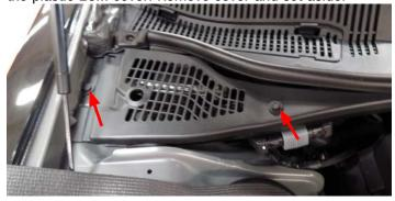
Dodge Charger/Chrysler 300: Using a panel puller, remove the five (5) push pins securing the passenger side of the plastic cowl.
