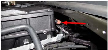
94. Connect the IAT extension harness to the stock IAT connector. Route the IAT extension harness behind the manifold and connect to the IAT sensor located on the rear research set the manifold.
