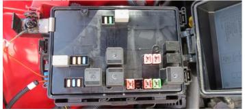
95. Open the fuse box and remove the fuse from location 6 (Ignition Coils/Injection 25A - See reverse of fuse box cover), this will be the front most fuse on most applications. Install that fuse in the bottom slot of the supplied fuse tap and the supplied 10 amp fuse in the top slot. Install the fuse tap in the slot previously occupied by the stock fuse.
