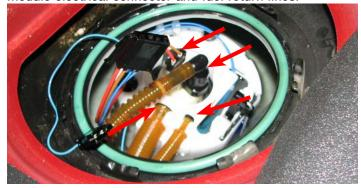
123. Carefully turn the fuel pump module on its side to drain the remaining fuel from the bottom reservoir and remove from the vehicle.
