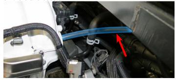
29. Carefully remove the intake manifold and set aside.
