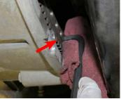
42. Using a 21mm socket and breaker bar, remove the factory crank bolt. Using the suppled crank bolt, install the drilling guide with the flat side facing outwards. Position drilling bushing in a comfortable position for drilling.
