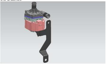
73. Mount the water pump/bracket assembly to the passenger side frame rail using the supplied M8 x 20mm bolts and M8 nuts from Bag #3. The pump will mount just below the radiator hose in front of the alternator.
