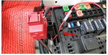
100. Mount the relay and fuse holder on the water pump harness on the metal tab with a wire tie.
