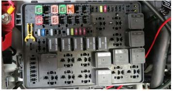
98. Open the fuse box and remove the fuse from location 39 (Power Steering / AC Clutch 10A - See reverse of fuse box cover). Install both supplied 10 amp fuses in the fuse tap. Install the fuse tap in the slot previously occupied by the stock fuse.
