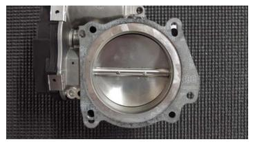
89. Reconnect the factory throttle body connector to the throttle body.
