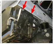
38. With the help from an assistant, carefully lower the radiator assembly and set aside.
