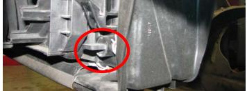
21. Remove the driver side PCV hose. Note that the 5.7L and 6.4L have different driver side PCV configurations.
