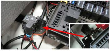
101. Route the water pump connector down to the electric water pump and connect it to the water pump.
