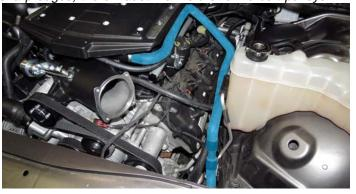
87. Attach the LTR to Manifold hose to the LTR and secure with a hose clamp from Bag #3. Apply two (2) pieces of convolute sleeve, about three (3) inches each, to the LTR hose as shown and secure with electrical tape or equivalent.
