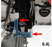
22. Loosen the worm clamps securing the air inlet tube to the airbox and throttle body. Disconnect the engine harness from the IAT sensor and remove the air inlet tube. Using a 8mm socket, remove the bolt securing the stock airbox and remove the airbox.
