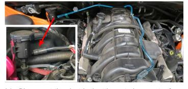
24. Disconnect the electric throttle control connector from the throttle body.
