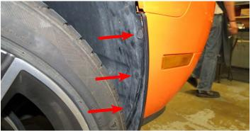
12. Use a 10mm socket to remove the bolts behind each front wheel well.
