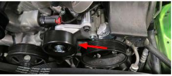
54. Use a 3/8" Fuel Line Removal Tool to detach the fuel input line from the factory hard line near the firewall on the passenger side. Attach the 90° end of the supplied fuel input line to the factory hard line.
