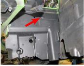
36. Using mechanic's wire or equivalent, securely hang the A/C condenser to the vehicle. Using an 8mm socket, remove four (4) bolts securing the A/C condenser to the radiator assembly.
