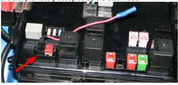
96. Use a 1/8" drill bit to drill a hole in the plastic rivet closest to the passenger side strut tower. Feed the bare wire extending from the water pump harness through the hole and insert it into the butt connector on the fuse tap. Crimp the butt connector firmly to secure the connection.
