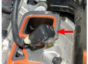
32. Using a 10mm socket, remove two (2) bolts securing each ignition coil. Remove the coils and note their order so that they can be reinstalled in the same order.
