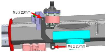
74. **2015+ Model Year Chargers Only:** Using the factory hardware, replace the existing bracket located under the passenger side headlight with the provided bracket to allow sufficient clearance for intercooler hoses.
