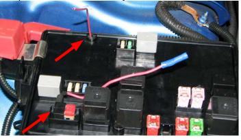
97. Tilt the fuse box up and remove the right nut. Mount the water pump harness relay on the protruding stud and reinstall the nut. Proceed to Step 100.
