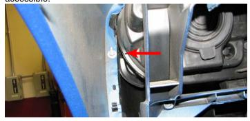
14. Carefully detach the sides of the front fascia and remove. Chrysler vehicles must also detach the top corners of the facia.
