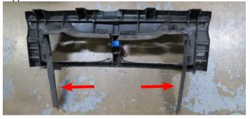
108. Using a Dremel or equivalent, grind down the lower tab on the passenger side of the front fascia support.
