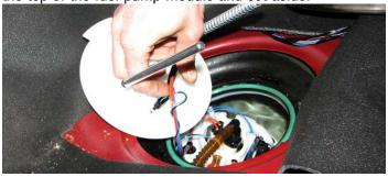
122. Press the quick connect release tab on the fuel supply line and remove. Now, disconnect the lower fuel pump module electrical connector and fuel return lines.
