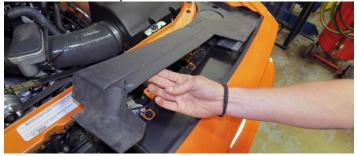
9. Dodge vehicles need to remove twelve (12) body pins, under the plastic radiator shroud, securing the fascia using a panel puller.
