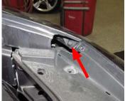
11. Use a panel puller to remove body pins securing the wheel well to the front fascia. Some vehicles use plastic rivets that need to be cut for removal. Pins are provided for reinstallation later.
