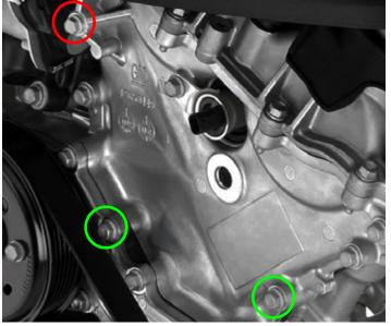
49. Attach the FEAD bracket and idler using the hardware provided in FEAD hardware bag #1 using blue Loctite.
