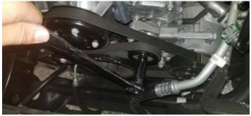
47. Disconnect the vacuum hose as pictured. Remove the bolts in the following picture and set aside. The bolts will be reused on the new bracket. The 13mm bolt has a nut on the opposite side. Be sure to recover this nut since it will be reused. Unplug and remove the vacuum assist pump and bracket from the front of the block, then remove pump from the OEM bracket.
