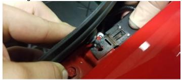
78. Replace the grill shutters by unbolting the LTR backets to the core support <u>on one side only</u>. Install the shutters back on and replace the bolts that were removed on that side. Once the grill shutters are tight on the one side, do the same for the other side. Doing this helps keep the LTR in place while you install the bolts. This makes it a lot easier to reinstall.
