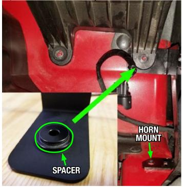
30. Replace the horn back into the same position on top of the forward water pump bracket strut using the same bolt that was removed. Reconnect the plug.
