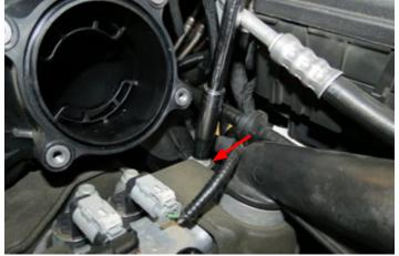
43. Once the manifold is removed, cover the intake ports to ensure nothing falls down into the ports.
