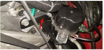
51. The new TMAP sensor is pre-installed from Edelbrock. A TMAP extension cable is included. Once the intake is installed, the TMAP will be difficult to access.
