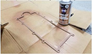
57. Place the gasket on the intake manifold base. Be sure to align the gasket with the holes to ensure a perfect seal.
