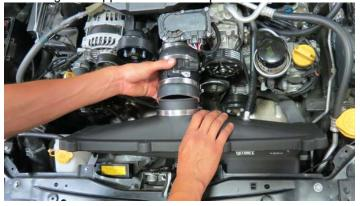
155. Clock the worm clamps to position the screws away from the A/C compressor belt/pulley. Double check that there is at least 6mm clearance between the coolant line on the throttle body and the belt on the AC compressor pulley.
