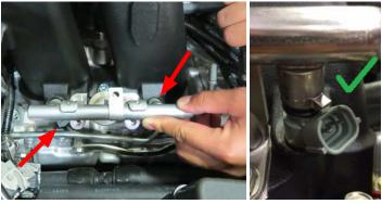
115. Connect the passenger side fuel crossover line to the fuel rail and engage the blue locking clip.
