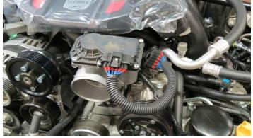
127. Using a factory hose clamp, secure the throttle body coolant outlet hose to the throttle body outlet fitting.
