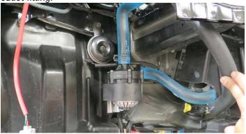
137. Route the water pump connector, from the previously installed water pump harness, down towards the water pump and connect it to the water pump. Secure the harness to existing wire looms and/or hoses.
