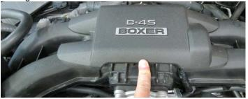
22. Unplug the MAP sensor connector located on top of the driver side intake manifold runner.
