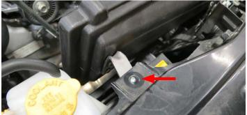
147. Use a M6 locknut and a M6 washer from Bag #4 to secure the front air box shroud to the isolator.
