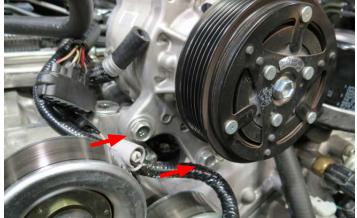
95. Using a 14mm socket, remove the rear A/C compressor bolt and carefully position the compressor forward. *NOTE: DO NOT remove the A/C lines as you will purge all of the pressurized freon.*
