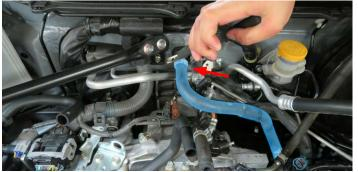
69. Using a hose cutter, or equivalent, cut approximately 1.75" from the passenger side heater hose.
