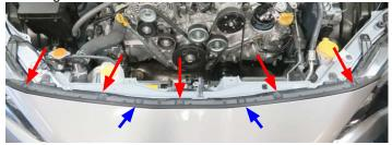
3. Remove the lower splash guard by removing three (3) bolts (green arrow) using a 10mm socket and nine (9) push pin rivets (red arrow) using a panel puller.
