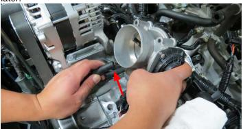
61. Remove the throttle body coolant hose from the coolant crossover using a hose clamp tool, or equivalent,.
