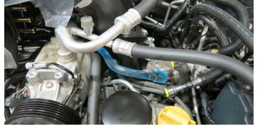
111. Realign the supercharger to the cylinder heads. Using two (2) M8 x 30mm bolts and one (1) M8 x 50 bolt, loosely secure the driver side runner to the cylinder head.
