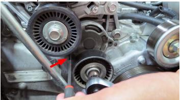
86. Using a 12mm and 14mm socket, remove the bolt securing the alternator to the alternator bracket and the bolt securing the alternator bracket to the engine.
