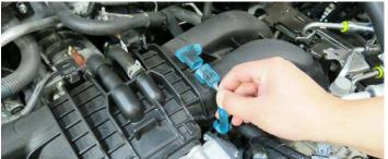
23. Disconnect the throttle body connector from the throttle body.
