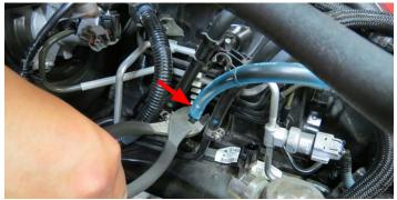
83. Connect the supplied 29" EVAP hose to the factory EVAP hard line. Route the hose towards the A/C compressor and under the driver side PCV hose. Connect the other end of the EVAP hose to the EVAP solenoid fitting farthest from the connector. Secure the EVAP hose to the solenoid using a 5/8" hose clamp from Bag #4.
