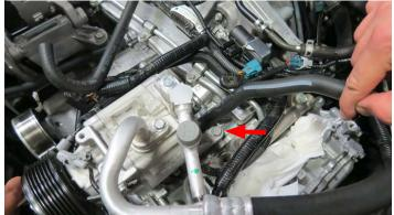
96. Using pliers, remove the driver side PCV hose located under the A/C compressor
