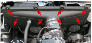
157. Connect the previously installed driver side PCV hose to the 1/2" barb fitting on the rear air box shroud.
