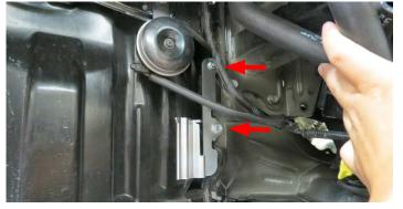
133. Using a 3/4" hose clamp from Bag #2, secure the LTR to W/P Hose to the top LTR fitting.
