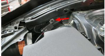
76. Route the Fuse Holder and Power +12V terminal, on the water pump harness, around the fuse box and towards the battery. Route the EVAP connector over towards the driver side cylinder head.
