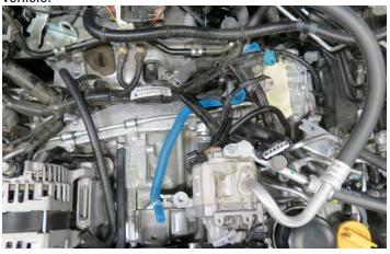
68. Using a hose clamp tool, or equivalent, remove the passenger side heater hose from the heater core fitting located on the firewall.
