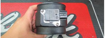
153. Using the worm clamps, secure the tapered coupler and the straight coupler to the MAF housing.
