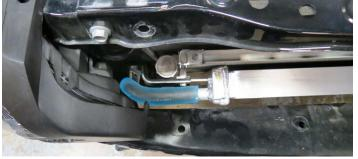
134. Route the W/P end of the hose down and over towards the water pump bracket.
