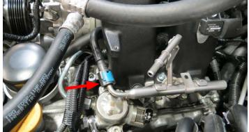
118. Connect the low pressure fuel feed line to the driver side fuel rail. Verify the lock is engaged by gently tugging on the fuel line.
