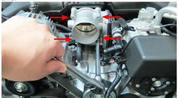
45. Using needle nose pliers, remove the engine harness from the rear passenger side manifold runner. Using a 12mm socket, remove three (3) bolts securing the passenger side of the manifold to the cylinder heads.
