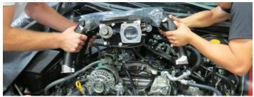
101. With the supercharger manifold properly positioned onto the cylinder heads, reinstall the A/C compressor and torque bolts to 22 ft lbs. TIP: The rear compressor bolt can be accessed through the opening of the driver side runner using a long extension and a universal socket.
