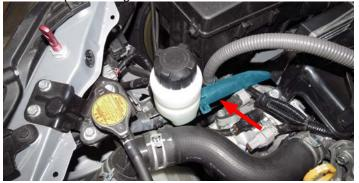
106. Using a 3/4" hose clamp from Bag #2, secure the 90° end of the Surge Tank **(Gen 1 tank shown)** to W/P hose onto the surge tank. Route the other end of the hose down towards the horn assembly along side the previously routed LTR hose.
