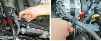
27. Remove all harness connectors from the ECU by depressing the locking tabs on the connectors and then rotating the connector levers outward until they release from the ECU.
