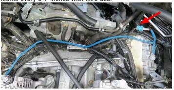
79. Using a 12mm socket, remove the bolt securing the brake booster hard line to the engine. Position the supplied EVAP bracket under the brake booster line and secure the EVAP bracket and brake booster line using the factory bolt.
