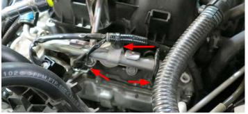
39. Using a 12mm socket, remove two (2) bolts securing the driver side fuel rail to the manifold. Remove fuel rail assembly and move aside.
