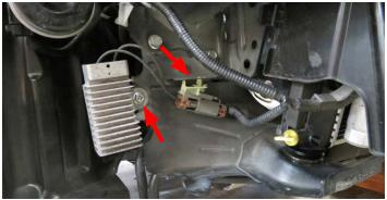
130. Using a drill and a 10mm drill bit, drill out the hole located on the crash beam support. Using a rivet nut tool, or equivalent, install the rivet nut from Bag #2 to the crash beam support.
