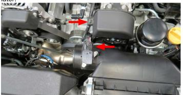
16. Using a 10mm socket, remove three (3) bolts securing the upper air box assembly and remove.
