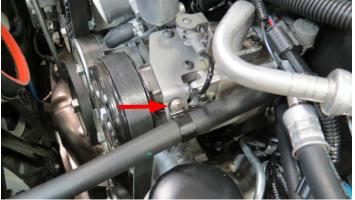
159. Connect the male MAF sensor connector, on the supplied TMAP harness, to the factory MAF sensor connector. Connect the female MAF sensor connector to the factory MAF sensor.
