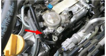
58. Install the low pressure fuel feed line onto the banjo fuel fitting. *TIP: Fuel line will be the one closest to the mechanical fuel pump.*
