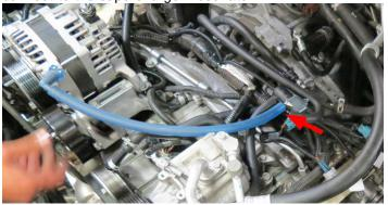
85. Rotate the tensioner clockwise using a 14mm socket. Insert a small screw driver into the grooves of the tensioner to hold it in position.
