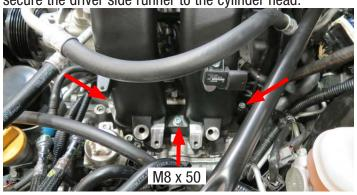
112. Using two (2) M8 x 30mm bolts and one (1) M8 x 50 bolt, loosely secure the passenger side runner to the cylinder head. Torque all six (6) bolts to 10 ft-lbs, starting with the center bolts and working outwards,
