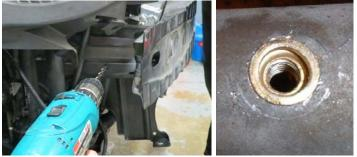
131. Secure the resistor to the rivet nut with the M5 x 20mm bolt from Bag #2. Secure the harness to existing vehicle harnesses as needed.
