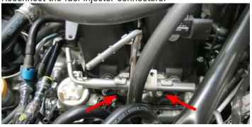
117. Connect the fuel crossover line to the driver side fuel rail and engage the blue locking clip.
