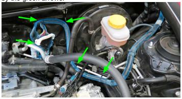
75. Mount the relay and ground strap on the water pump harness to the chassis bolt adjacent to the fuse box.
