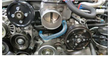
128. Using a 14mm socket, rotate the belt tensioner clockwise and install the supplied drive belt using the routing diagram below.
