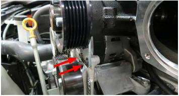
121. Connect the 45° end of the previously installed EVAP hose to the top nose fitting. Connect the RH/Passenger PCV to the bottom nose fitting. Manual applications will connect the Brake Booster hose to the center nose fitting. Automatic applications will remove the fitting plug from the stock intake manifold and install it to the center nose fitting.
