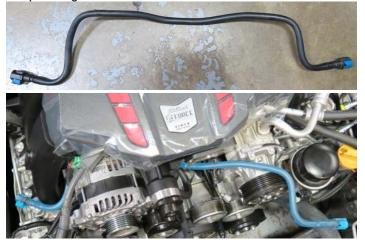
110. Snake the other end of the fuel crossover behind the A/C compressor and out in front of the driver side runner.
