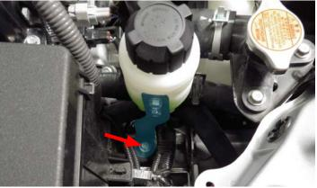
108. Using two (2) M6 x 10mm bolts from Bag #2, secure the surge tank to the surge tank bracket.
