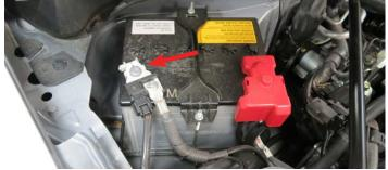
Using a 10mm socket and a panel puller, remove five
