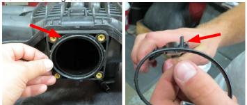
124. Install the O-ring seal onto the supercharger throttle body flange. Connect the throttle body coolant inlet hose to the inlet fitting and secure with the factory hose clamp.
