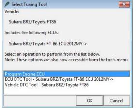
18. The ProECU Programming Tools window will only be displayed if ProECU successfully established a connection to the ECU. Proceed to Step 20 if you have established a successful connection. If not, please proceed with the cautionary notes.
