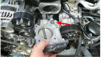
125. Using the factory throttle body bolts, secure the throttle body to the supercharger with the connector oriented upwards.
