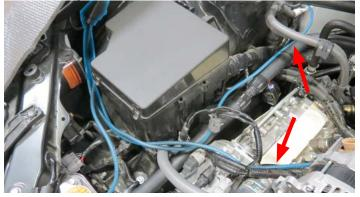
77. Connect the +12V Constant Power terminal to the positive stud on the battery terminal. Secure the Fuse to existing wire looms with wire ties.
