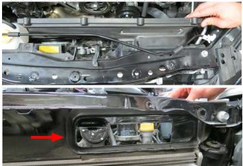
145. Use the M6 x 16mm Hex Flange bolt from Bag #4 to secure the front air box shroud to the upper radiator support. This is done from the inside of the air box by threading the bolt through the welded nut on the radiator support.
