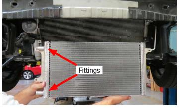
93. Align the A/C condenser and the LTR. Using a 10mm socket, secure the LTR to the A/C condenser using the factory hardware.
