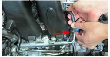
116. With the fuel injectors securely positioned on the driver side fuel rail, carefully install the fuel rail assembly with the injector connectors oriented outwards. Secure the fuel rails with the factory bolts and torque to 10 ft-lbs. Reconnect the fuel injector connectors.
