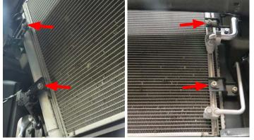
92. Remove the protective covers on the Low Temp Radiator (LTR) fittings. Carefully position the LTR, with the fittings pointing towards the passenger side of the vehicle, onto the A/C condenser mounting brackets.
