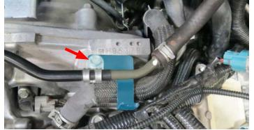
80. Remove the EVAP solenoid from the bottom of the factory intake manifold.
