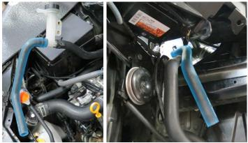
107. Using a 10mm socket, remove the bolt securing the front of the fuse box. Insert the surge tank bracket under the fuse box and secure the bracket along with the fuse box with the factory bolt.
