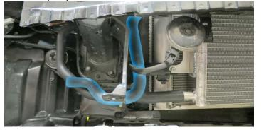
135. Install the supplied water pump onto the water pump isolator and install the assembly onto the water pump bracket. Clock the water pump so that the outlet fitting is perpendicular to the body and pointing towards the driver side of the vehicle.
