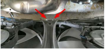
140. Install the isolator onto the lower air box support bracket. Using a 10mm socket, remove the bottom bolt securing the hood latch assembly and install the supplied lower air box support bracket using the factory bolt.
