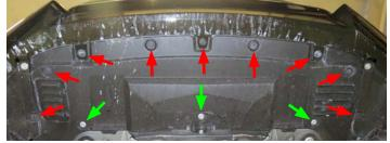
4. Using a 10mm socket, remove three (3) bolts securing the splash guard/fascia support.
