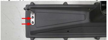
143. Install the supplied 5/16" grommet and grommet spacer onto the air duct of the front air box shroud.
