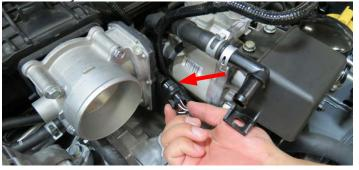
24. Remove the PCV and brake booster hoses attached to the top of the intake manifold. *NOTE: Automatic applications will have a PCV hose and a rubber cap.*
