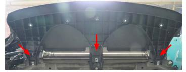
5. Use a panel puller to remove two (2) push fit rivets (red arrow) and a 10mm socket to remove two (2) bolts (green arrow) securing the fascia to the outer splash guards.
