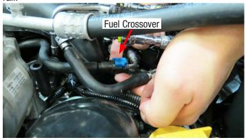
38. Unplug the driver side fuel injector connectors. Using needle nose pliers, remove the plastic rivet securing the injector harness to the fuel rail.
