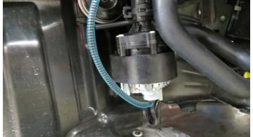
138. Using a 12mm socket, loosen four (4) bolt securing the top radiator support.
