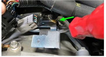
74. Relocate the transmission plugs and harness behind the heater hoses. Secure the harness and plugs to existing engine harnesses and A/C lines with wire ties as designated by the green arrows.
