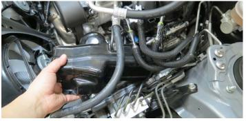
37. Release the blue locking clip from the fuel crossover and disconnect the crossover line from the driver side fuel rail.
