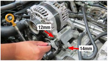
87. Position the supplied FEAD bracket onto the alternator mounting bracket. Using the M10 x 70mm bolt from Bag #1, loosely secure the FEAD bracket to the lower alternator bracket bolt provision.
