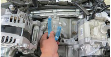
62. Install the straight end of the supplied throttle body inlet hose to the coolant crossover and secure with the factory hose clamp.
