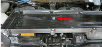
148. Re-secure the top radiator support using the factory hardware.
