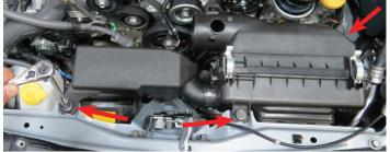
17. Using a 10mm socket, remove two (2) bolts securing the lower air box assembly and remove.
