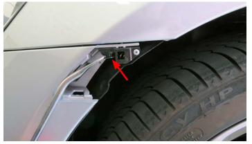
9. Unplug any front fog lights, if applicable, and carefully remove the front fascia.
