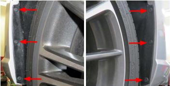
7. Carefully remove both side marker lenses by gently pulling out the upper corner of the lenses. Unplug the bulb assemblies and remove. *Tip: Lenses are secured with three (3) metal clips pointed out by the red arrows.*
