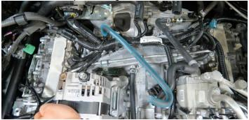
65. Using long needle nose pliers, remove the throttle body outlet coolant line from the driver side cylinder head fitting.
