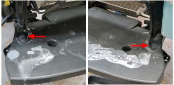
11. Connect a rubber hose to the drain barb located on the petcock. Place the other end of the hose into a drain bucket and loosen the petcock to drain the radiator fluid. *TIP: Rubber hose is not require but will limit spillage and cleanup.*
