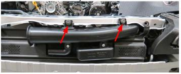
18. Using a panel puller, remove six (6) push pin rivets securing the radiator shroud and remove.
