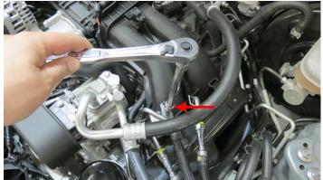
33. Disconnect the rubber EVAP hose from the EVAP hard line.
