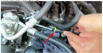
43. Using pliers, remove the rubber EVAP line from the hard line assembly.
