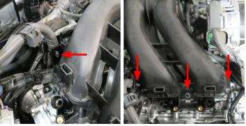
46. Using a 12mm socket, remove three (3) bolts securing the driver side manifold to the cylinder heads.
