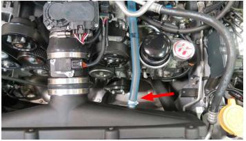
158. Using the 3/4" Hose Clamp and M5 x 8mm Button Head Flange bolt from Bag #4, secure the driver side PCV hose to the PCV support bracket.
