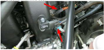
161. Using the push mount zip tie from Bag #2, secure the TMAP harness and the throttle body extension harness to the PCV support bracket.
