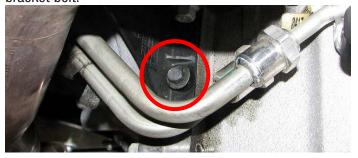
95. Use a 13mm socket to remove the two starter bolts.
