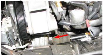
75. Use a 6mm Allen tool to hold the tie rod ball stud stationary while using an 18mm wrench to loosen the nut.
