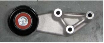
135. Use a 10mm socket to remove the three bolts on the
