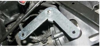
157. Re-install the horns using the OE nuts. Be sure to orient the horns so as to allow a little bit of slack in the horn's wiring harness. *Warning:* Do not mount the horns with the opening facing up, as they will accumulate condensation and cease working.
