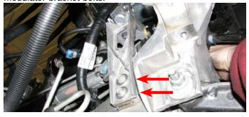
88. Use an 18mm socket to remove the two steering rack nuts and bolts.
