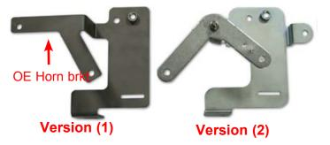
156. **NOTE:** This step only applies to customers who received version (1) of the water pump brackets. Install the supplied stand-off and lock nut onto the OE horn bracket. Proceed by mounting that assembly, with the supplied M6 x 10mm bolt, to the water pump bracket as shown below.
