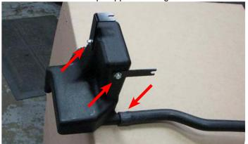
169. Use a 10mm socket to install the brackets supplied in Bag #2 on the reservoir. The image above shows the installed orientation.
