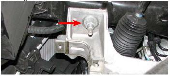
84. Disconnect the ride height sensor electrical connector from each side, if equipped.
