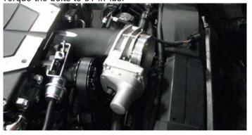
217. Connect ETC harness to the throttle body motor.
