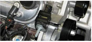
142. Use a 15mm wrench to remove two bolts retaining the power steering reservoir bracket. Use a pair of pliers or hose clamp tools to disconnect the lower reservoir-to-pump hose. Note that it is not necessary to fully remove the reservoir from the engine.
