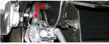
163. Lower the heat exchanger hose assembly along the driver side of the radiator shroud.
