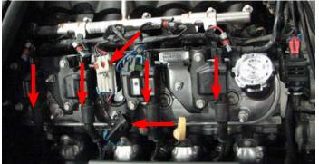
37. Use a 10mm socket to remove the five bolts retaining the coil bracket on each valve cover then remove both coil bracket assemblies
