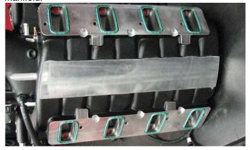
178. Install supplied Manifold to EVAP Solenoid Hose on manifold fitting below hub snout.
