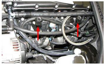
206. Tuck the wire harness tight against the fuel rails. Verify nothing will be pinched or damaged when the coil covers are installed.
