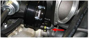
195. Route the other end of the PCV hose to the tube extending from the valley plate and attach it.
