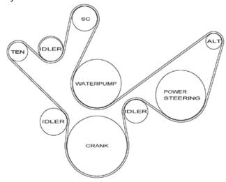
211. Use a breaker bar and a 16mm socket to push the tensioner enough to get the belt on, then double check the routing.
