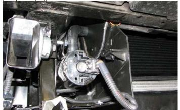
161. Plug the male connector on the T-segment of the harness into the EVAP solenoid then plug the factory EVAP connector into the female connector on the T-segment.
