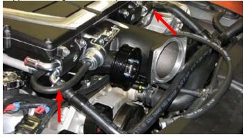
193. Clip the heat exchanger hose assembly to both lower fittings at the front of the supercharger manifold.
