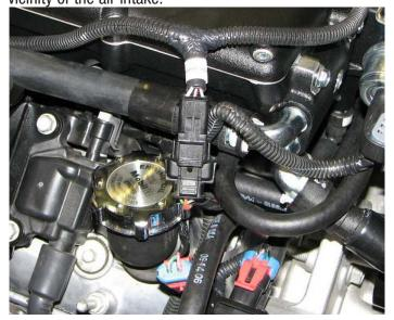
209. Remove the upper radiator hose to install the serpentine belt.
