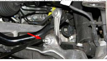
78. Use a 13mm socket to remove the four bolts retaining the stabilizer brackets.
