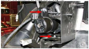
NOTE: There are two different water pump brackets: Version (1) requires the use of your OE horn bracket. Version (2) has an integrated horn bracket. You should have received one of the two brackets; If your supercharger kit includes bracket version (2), you may disregard Step 157.
