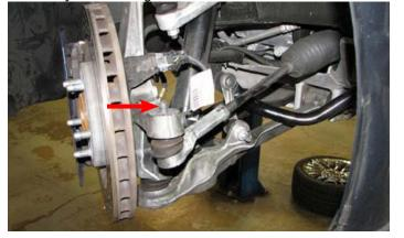
76. Use GM Ball Joint Separator #J 42188 to separate the steering knuckle from the tie rod ball stud then remove the tool and the nut. Use this procedure for both sides.
