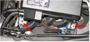
167. Use a 7mm socket to remove the fuse box bolt located in the passenger side fender well.
