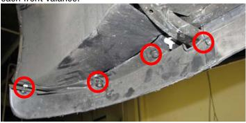
23. Remove the five 7mm and two 10mm nuts retaining the fascia from below.
