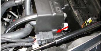
160. Route the intercooler water pump wire harness extending from the relay down to the intercooler water pump and plug in the connector.
