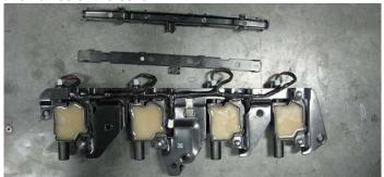
199. Tuck the fuel injector wiring harness and the EVAP Solenoid to Firewall Fitting Hose between the valve cover and manifold then use a 10mm socket and the ten stock bolts to install both coil brackets on to the valve covers.
