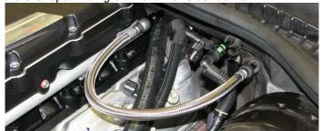
197. Connect fuel injector electrical connectors.
