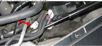
175. Reinstall the fender well fuse box bolt.
