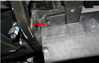
155. Use a 10mm socket to install the pump bracket using the M6 x 45mm bolt and M6 nut on top and the M8 x 30mm bolt on the bottom, all supplied in Bag #2.
