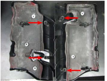
203. Install the stock grommets into the coil cover brackets supplied in Bag #6.
