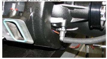
179. Clear engine valley of any hoses, wires, tools, etc. Lay the intercooler-to-reservoir tank hose in the engine bay, routed along the firewall behind the oil pressure sensor, and connect it to the intercooler reservoir inlet, securing the fitting with a hose clamp supplied in Bag #2.
