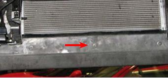
150. Use a 10mm socket to install the heat exchanger, using the 20mm bolts supplied in Bag #2 on the side, and the stock air dam bolt on the bottom.
