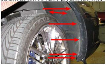
18. Pull back the inner fender well to access the two bumper studs on each side. Use a 10mm deep socket to remove the nuts.
