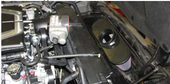
223. Use a T15 Anti-Tamper Torx driver to remove the MAF sensor from the stock airbox.
