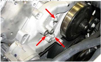
136. Use a 2" long 6mm Allen socket and the three 90mm bolts supplied in Bag #1 to install the lower idler bracket on
