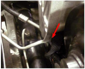
137. Use a 15mm socket and the two stock bolts to mount the new tensioner bracket onto the water pump then torque them to 37 ft-lbs.
