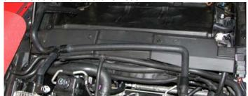
164. Connect the heat exchanger hose assembly to the heat exchanger through the hole drilled in the shroud. Secure the fitting with a hose clamp supplied in Bag #2.
