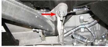
91. Insert a pry bar between the frame and front driver side cradle mount.
