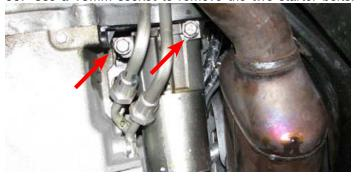
96. Disconnect electrical connector at top of starter.
