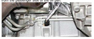
94. Use a 10mm socket to remove the starter support bracket bolt.
