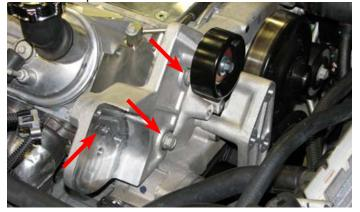
139. Apply blue loctite to the threads of a 20mm bolt supplied in Bag #1, then use a 12mm socket and the supplied washer to mount the pulley on the tensioner bracket and torque it to 18 ft-lbs.
