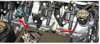
202. Remove the grommets from the stock coil covers.
