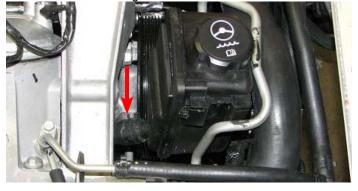
143. Slide the old bracket off the reservoir then install the supplied bracket using a 15mm socket and the stock bolts. Slide the power steering reservoir onto the new bracket and reattach the lower reservoir to pump hose.
