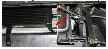
165. Connect TMAP harness to TMAP sensor near rear of manifold.
