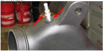
221. Install the hose barb supplied in Bag #5 into the new air inlet tube.
