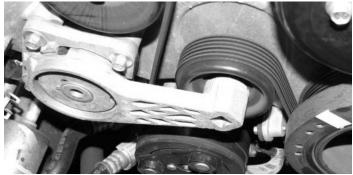
3. Place the tensioner in a cloth wrapped vice and use a grinding wheel or hacksaw to remove the stop.
