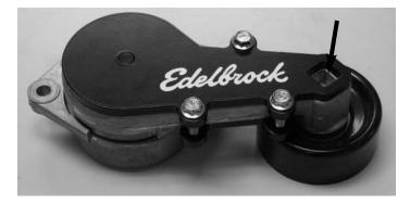
6. Use a 10mm socket to reinstall the tensioner.
