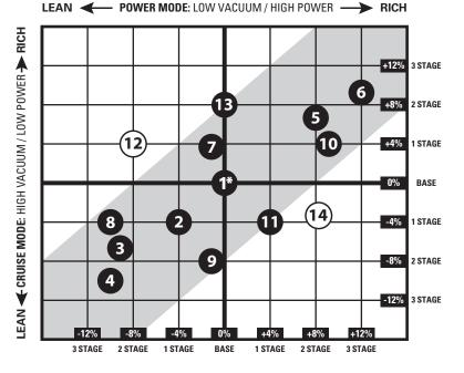
**STEP 1** Select the Calibration Reference Number that is nearest to your desired combination of *Cruise Mode* and *Power Mode*.
