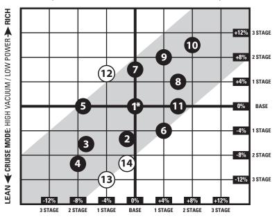
**STEP 1** Select the Calibration Reference Number that is nearest to your desired combination of *Cruise Mode* and *Power Mode*.
