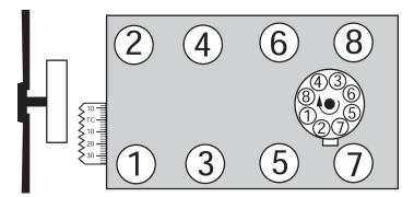
Figure 1 - 396-454 C.I.D. Chevrolet V8 Firing Order and Timing Marks Firing Order: 1-8-4-3-6-5-7-2 Turn distributor counter clockwise to advance timing
