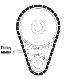
Figure 2 - Timing Chain Sprocket Alignment
