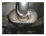
5) Place a provided clamp onto the outlet of one of the **#952546** mufflers, then place the muffler onto the back of the left over-axle pipe with the inlet of the muffler toward the center of the vehicle. Rotate the muffler so that it's level and support with a stand. Tighten the clamp on the outlet enough to hold but still allow for adjustment. Repeat this step with the other muffler on the right side of the vehicle.
