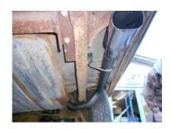
3) Place the left side exit pipe **#86148** up into place and connect the hanger at the rear of the pipe to the rubber mount installed in step 1 above. Slide the hanger into the rubber mount until about <sup>3</sup>/<sub>4</sub>" of the wire hanger sticks out from the rear of the rubber mount. Repeat this step on the right side of the vehicle with exit pipe **#86147**.
