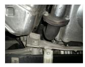
2) At the front of each of the muffler/over axle pipe assembly there is a two bolt flange. Using a 15mm wrench loosen the nuts and remove the bolts from these connections. Retain the hardware; it will be used for the installation of the Flowmaster system.
