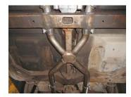
1) After installing either the **81101** or **81103** downpipe kits, place a provided 2.50" clamp onto the expanded ends of X-pipe assembly **86233S**, then slide onto the back of the manifold pipes, be sure that the pipes are fully slipped together. Place a stand under the rear of the assembly and tighten the clamps enough to hold, but still allow for adjustment. The Flowmaster embossed side of the assembly will be facing the ground.
