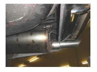
Place one of the supplied **HA602** rubber mounts onto the wire hanger of left muffler assembly **842557-356**. Place a provided clamp onto the muffler inlet, then place the assembly onto the back of the mid pipe and slide the two fully together. Support the muffler with a stand. Using a supplied 3/8" bolt, nut, washer and lock washer, bolt the **HA602** hanger to the hole in the frame above the muffler outlet.
