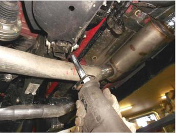
Begin by measuring back  $1\frac{1}{2}$ " from the rear of the suspension cross-member shown in the photos above and make a mark on both pipes. Support the exhaust system both in front and behind the area to be cut, then once you've double checked that the measurements are correct, cut both pipes at the marks. **Note: Use caution when cutting!**
