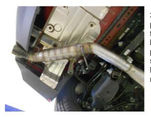
3) Adjust and level the two muffler assemblies to provide a satisfactory fit. They can also be adjusted forward or back to get the desired position in the rear bumper cut-outs. A minimum of 1/2" clearance around all parts of the system must be maintained; while keeping suspension travel and vibration in mind. After adjustments have been made, and you are satisfied with the fit, you may now securely tighten the two muffler inlet clamps.
