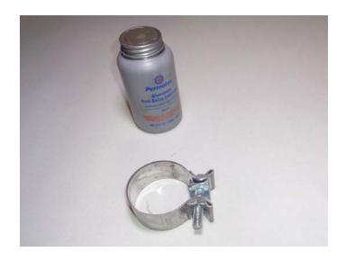
Place clamp (MC300BS) onto slip-fit of muffler (815430-517). Push wire hangers on muffler into rubber isolators and connect to factory tailpipe inlet. Tighten clamp just enough to allow for adjustment.
