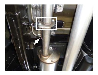
5. Remove muffler wire hangers from mounts, then remove cut out muffler section from factory exhaust system. Remove gasket from factory muffler inlet and retain for re-use.
