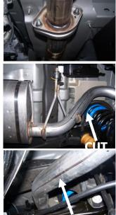
**1.** To remove the stock exhaust, remove it from the two bolt flange in front of the muffler. Do not throw away you will re-use bolts. Disengage the welded hangers using WD-40 from the OEM rubber grommets. Do not damage or remove the rubber grommets as you will reuse them to mount your new system. Now, cut off tailpipe before and after rear axle for removal.
