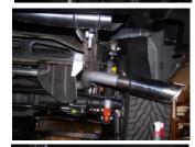
**8.** Install the exit pipes #E. Use clamp #G to secure exit pipes to tailpipes. DO NOT TIGHTEN. Reinstall spare tire. Use zip ties to secure brake, gas lines as necessary.
