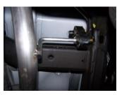
**5.** Remove spare tire to install tailpipes. Now install passenger side tailpipe #D into the muffler 1<sup>1</sup>/<sub>2</sub>-2". Use clamp #G to secure tailpipe to muffler. DO NOT TIGHTEN. Insert welded hangers into rubber grommets.
