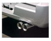
Install the stainless tips. Clamp down. To clean your stainless tips use any stainless cleaner or a Scotch Brite pad. Now go back and tighten all clamps, nuts and bolts. Start from the front and work back.
