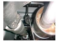
Lay out the exhaust on the floor so it looks like the drawing and compare parts with manual. To remove the stock exhaust un-clamp it just in front of the muffler. Leave all rubber grommets in place. Use WD-40 to aid in removal of exhaust and the hangers.
