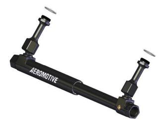
5. With the fuel log in place pivot the log to the position that provides the most clearance and tighten the pivot nuts to 20 in-lbs.
