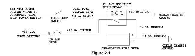
Note: Route all electrical wires clear of any moving suspension or drivetrain components and any exhaust components! Protect wires from abrasion and road obstructions or debris.
