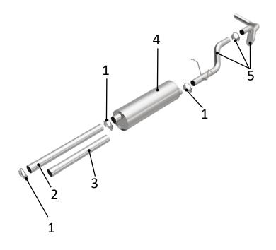
2: 155" WB 3: 138" WB (Carefully read all instructions before installation) Disconnect the vehicle's battery before removal of the OEM exhaust system. This will prevent electrical accidents and will reset the computer if it applies to the vehicle. Remove existing exhaust system from the vehicle. Only remove parts that will be replaced. Clean existing flange with a wire brush to ensure proper sealing.
