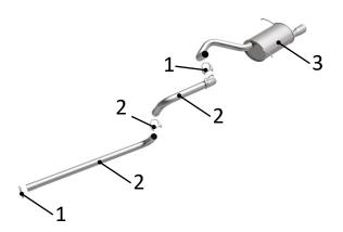
(Carefully read all instructions before installation) Disconnect the vehicle's battery before removal of the OEM exhaust system. This will prevent electrical accidents and will reset the computer if it applies to the vehicle. Remove existing exhaust system from the vehicle. Only remove parts that will be replaced. Clean existing flange with a wire brush to ensure proper sealing.
