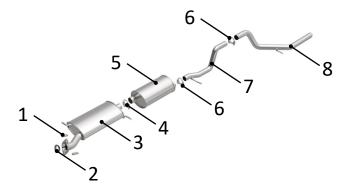
(Carefully read all instructions before installation) Disconnect the vehicle's battery before removal of the OEM exhaust system. This will prevent electrical accidents and will reset the computer if it applies to the vehicle. Remove existing exhaust system from the vehicle. Only remove parts that will be replaced. Clean existing flange with a wire brush to ensure proper sealing.
