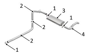
(Carefully read all instructions before installation) Disconnect the vehicle's battery before removal of the OEM exhaust system. This will prevent electrical accidents and will reset the computer if it applies to the vehicle. Remove existing exhaust system from the vehicle. Only remove parts that will be replaced. Clean existing flange with a wire brush to ensure proper sealing.
