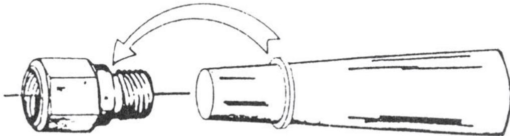
**Note** Slide pressure hose fitting back and remove old seal. Soften new seal in warm water, expand over a tapered punch, then transfer to hose as shown.
