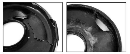
Typical vacuum booster diaphragm failure due to gas or gasoline fumes
