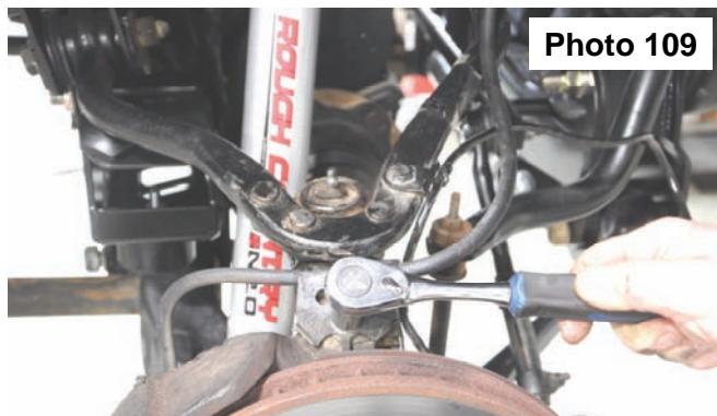
Install brake line on knuckle.
