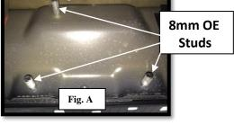
Step 5: Staring with the rear bracket, push up towards the pinch weld so the 3" main bar is as high and tight to the body as possible. Tighten all three 8mm flanged nuts.
