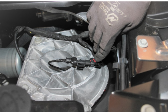
If your vehicle is equipped with Magnoride, disconnect the plug at the top of the shock tower.
