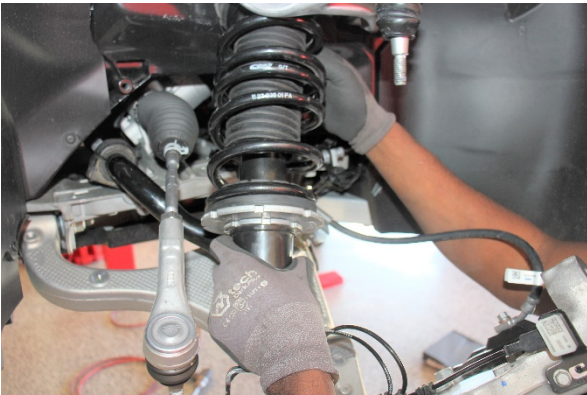
Remove the driver's side strut assembly.
