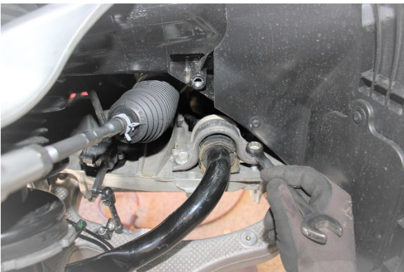
Loosen and remove the 15mm sway bar bracket bolts from both sides.
