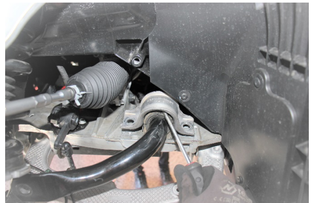
Remove the sway bar brackets.
