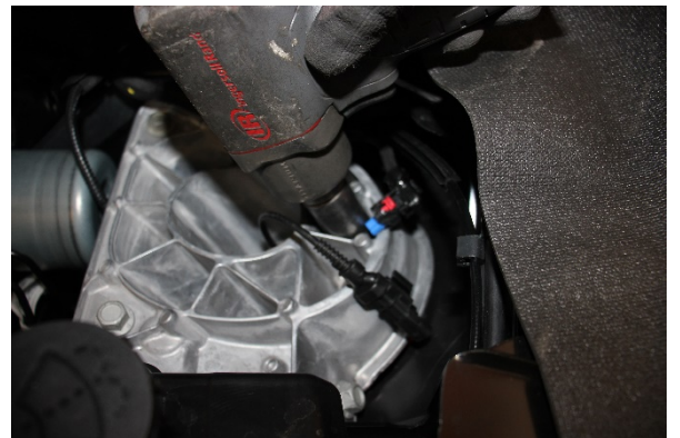
Loosen and remove the 13mm bolts at the top of the shock tower.
