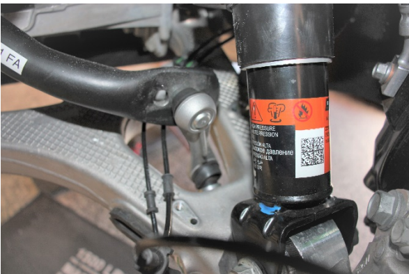
Install the end link to the sway bar in the desired hole position.
