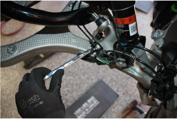
Begin by removing the wheel speed sensor bracket from both sides of the vehicle.
