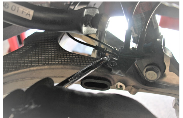
Reinstall the wheel speed sensor bracket.
