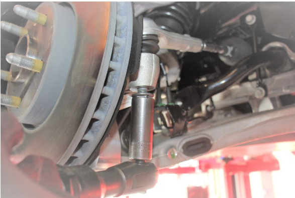
Remove the tie rod from the driver's side.
