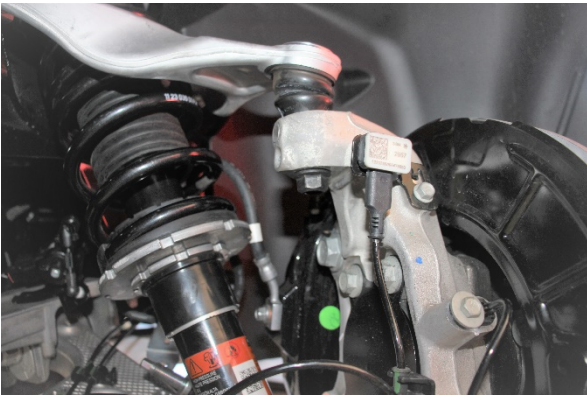
Reinstall the upper control arm to the steering knuckle
