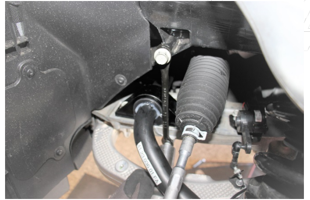
Reinstall the under body brace.
