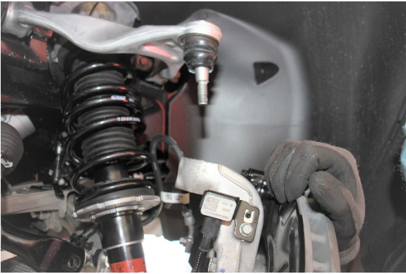
Loosen and remove the upper control arm from the steering knuckle.
