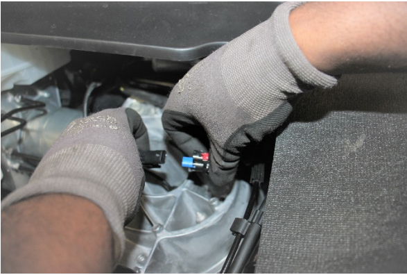
Reinstall the Magneride connector, if equipped, and tighten the upper shock tower bolts.
