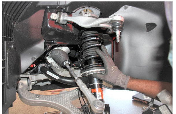
Reinstall the strut assembly.
