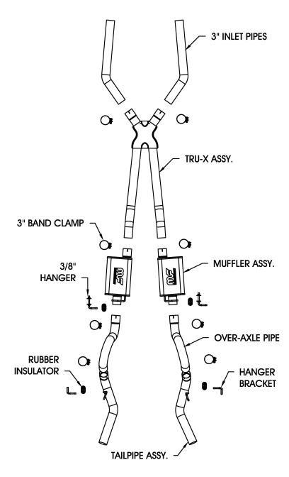
**Note:** This system is designed to work with OEM-style exhaust manifolds, or tubular headers. Due to the various applications possible, some modification and welding is required for a proper fit and finish.
