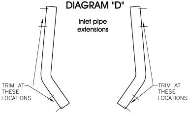
**Note:** This system is designed to work with OEM-style exhaust manifolds, or tubular headers. Due to the various applications possible, some modification and welding is required for a proper fit and finish.
