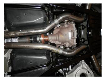
**Step 2.** Begin installation of the new system by attaching both Inlet Pipe Assemblies to the pipes you have just cut. Loosely secure using the supplied 2.50" clamps. Engage the welded hangers to the rubber insulators. Leave all clamps loose until final adjustment.
