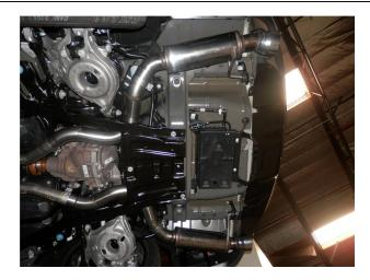
**Step 3.** Next attach both Muffler Assemblies to the Inlet Pipe Assemblies using the supplied 3.00" clamps and fitting the hangers into the rubber insualtors.
