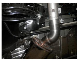
**Step 4.** Begin installation of the new system by sliding the D/S Muffler Assembly inlet onto the cut outlet of the OEM exhaust and loosely fasten with the supplied 2.75" clamp. Fit the hangers into the rubber insulators.
