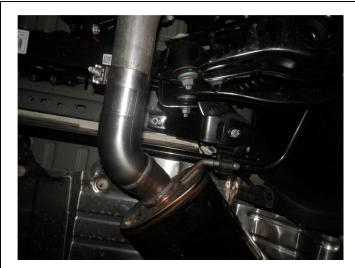
**Step 5.** Install the P/S Muffler Assembly in the same manner. Leave all clamps loose for final adjustment of the system.
