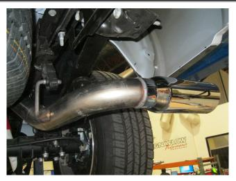
Step 4. Next loosely attach the Tailpipe Assembly to the Muffler Assembly using the supplied clamp. Engage the welded hanger to the rubber insulator.
