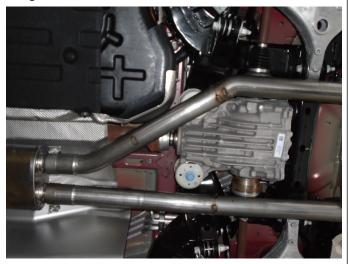
Step 4. Install the new Mid Pipes to the Muffler Assembly using the supplied clamps. Engage the welded hangers to the rubber insulators.
