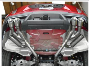
Step 5. Install the new Tail Pipe Assemblies to the Mid Pipes using the supplied clamps. Engage the welded hangers to the rubber insulators.
