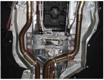
Step 2. Install your new system by first attaching the new Inlet Pipes to the catalytic converter outlets using the supplied clamps. Keep all clamps loose to allow for final adjustment.
