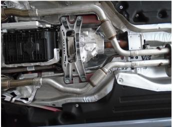
Step 1. Remove the OEM system by first loosening the clamps attaching the stock muffler to the Inlet Pipes. Next loosen the clamps attaching the Inlet Pipes to the catalytic converters. Next, Disengage all welded hangers from the rubber insolators. The exhaust system can now be removed. Retain all fasteners and insulators as they will be needed to mount your new MAGNAFLOW system.
