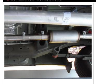
Step 5. Install 12" Extension Pipe if vehicle is 6.5' Bed. If not, disregard this step.
