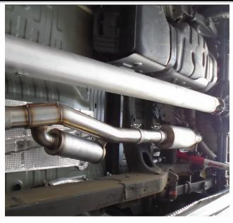
Step 7. With the new MAGNAFLOW system in place all loose band clamps can now be tightened. Your installation is complete.
