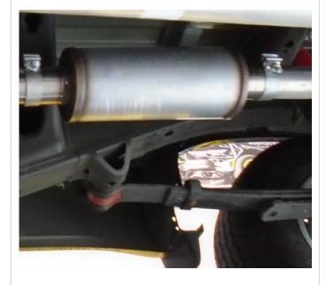
Step 6. Slip the Outlet Resonator exit pipe over the cut OEM rear pipe. Loosely secure using the supplied band clamp. Engage the welded hangers to the rubber insulators.
