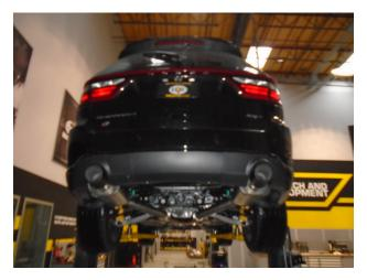
**Step 5**. Once a final position has been chosen for the new exhaust system, evenly tighten all clamps and fasteners using the torque specifications on page one of the instructions. Inspect all fasteners after 25-50 miles of operation and re-tighten as necessary.
