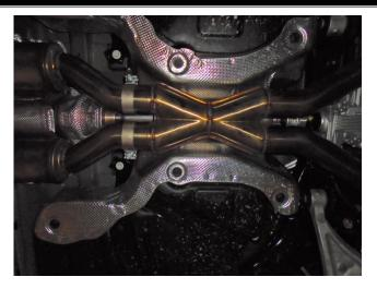
**Step 3.** Next attach the X-Pipe Assembliy to the Resonators using the supplied 3.00" clamps
