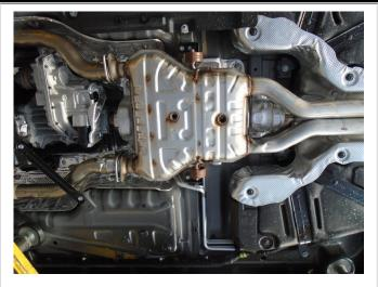
**Step 1.** Remove the OE exhaust system by first loosening the spring bolt fasteners from the flanges located at the front of the underbody Resonator. Next working front to rear extract the hangers from the rubber insulators and remove the complete exhaust system. Retain insulators as they will be used to install the new system.
