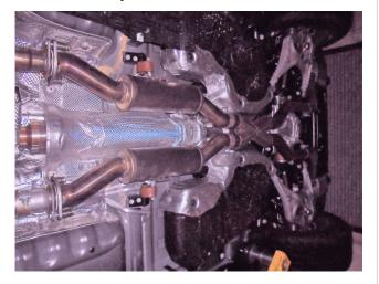
**Step 2.** Begin installation of the new system by loosely attaching the Driver and Passenger side Resonator assemblies the the two bolt flanges using the OE spring bolt fasteners and fitting the hangers into the rubber insulators. Leave all clamps and fasteners loose until final adjustment.
