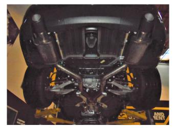
**Step 4**. Finish by installing the Passenger and Driver Side Muffler Assemblies using the suppled 3.00" clamps and fitting the hangers into the rubber insulators.
