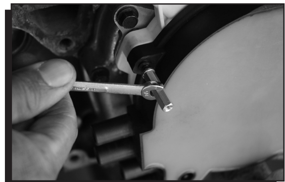
Figure 7 Removing the Original Cap.
