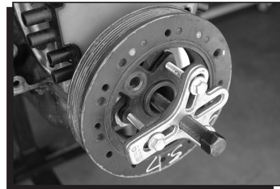
Figure 5 Removing the Hub.
