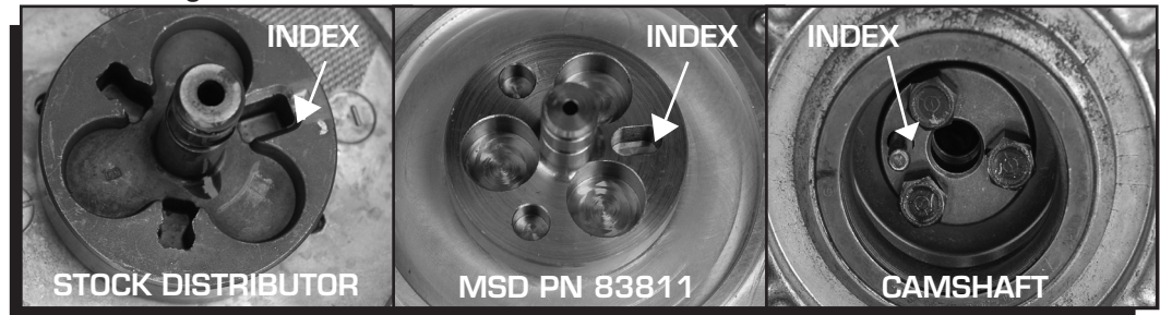
Figure 1 The Drive Mechanism of the PN 83811 Distributor.
