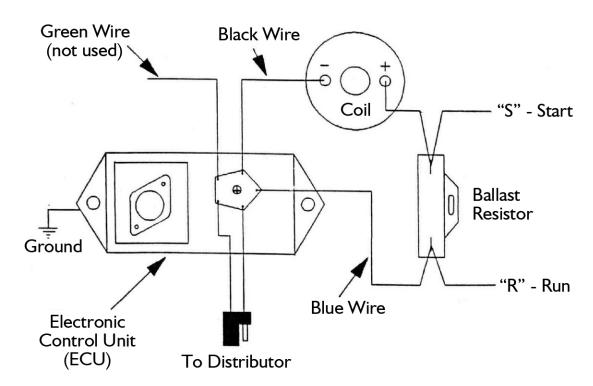
Typical Wiring Diagram for "Street Rod" Installation
