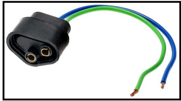
The factory, 2-wire regulator connector from the harness needs to be used. Due to a lack of usage by most customers, these connectors are not included with this Painless chassis harness. If you do not have these connectors, they can be obtained online, at a local auto parts store.
