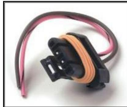
Without this resistance, the regulator on the alternator will burn up. A resistor, splices, and heat shrink, seen on [page 52](#), are provided in the "ALTERNATOR" bag kit. The resistor simply needs to be installed inline on the pin "L" wire, **#914**, as shown in the diagrams on the next page.
