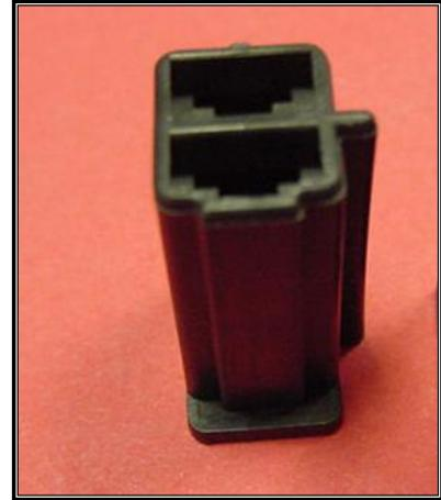
Re-use the connector from the factory harness, seen to the right, or use the small insulated terminals that have been provided in the parts kit. It does not matter which tab each wire connects to. Once connected to the switch, route the cutoff portion of **#919** to the "S" terminal on the Starter and connect as mentioned on the previous.
