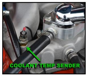
• Route this LT. GREEN #921 wire to the coolant temp sensor, cut to length, strip 1/4" insulation, and crimp on the appropriate terminal for your connection, and connect.
