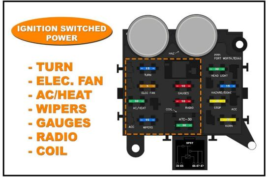
The drawing above shows all the switched ignition fuses. These fuses are powered by wires coming from the ignition switch (wires **#931**, **#932**, and **#933**) and receive power depending on what position the ignition switch is in. <u>NONE OF THESE FUSES SHOULD</u> <u>HAVE POWER WHEN THE IGNITION IS IN THE OFF POSITION.</u> The <u>Ignition Switch</u> <u>Section</u> beginning on page 89 of this manual will go into further detail about power supplied to these fuses.
