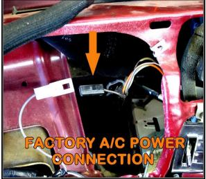
• Locate the inline connector on the factory heat or A/C harness, it will be a single-pin connector on a wire several inches away from the blower switch connection. Connect the **BLACK/WHITE #904** power wire to this wire on the air conditioning harness.
