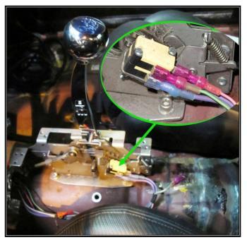
700-R4, TH200, 200-4R, & 4L60 transmissions. This part can be used as either a reverse switch or a neutral safety switch.
