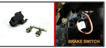
applied. This is usually the pair of terminals closest together. These pins are for cruise control and/or torque converter lockup.
