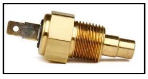
The coolant temp sending unit or temp switch can be mounted in the intake manifold or in the side of either cylinder head. These will have a peg, tab, or threaded post to connect to, as seen in the photos on this page. Terminals have been provided for those with the style of sensor seen below. Your factory notched connector will need to be re-used; rollover crimpers will be needed to properly install this terminal.
