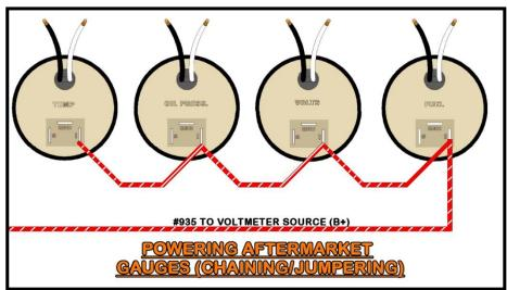
Grounds need to be supplied to the gauge lights and to any ground tab on the gauges. The installer needs to run their own ground circuit for gauge connections. To make these ground connections you can splice from the installer provided ground wires to all the gauges or chain/jumper it all together. Both methods can be seen in the following two drawings:
