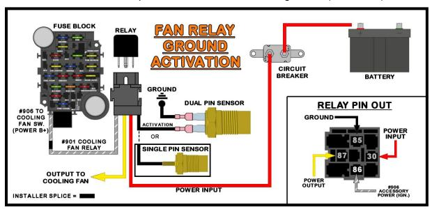
IF A TOGGLE/ROCKER SWITCH IS BEING USED WITHOUT A RELAY, MAKE SURE THE AMPERAGE OF THE COMPONENT YOU ARE POWERING DOES NOT EXCEED THE CAPABILITIES OF THE SWITCH OR SWITCH FAILURE WILL OCCUR. IF YOU NEED A RELAY KIT PAINLESS OFFERS PART #'S 30128, 30128, & 30130.
