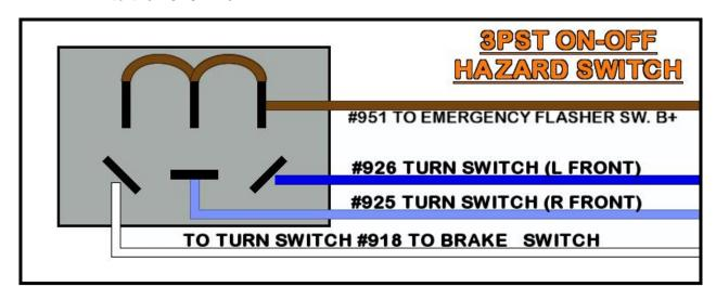
Also, a simple SPST On-Off switch can be used to flash only the brake lights in the event of an emergency. This diagram will not flash the front turn signals like a traditional hazard flasher which your local laws may require.
