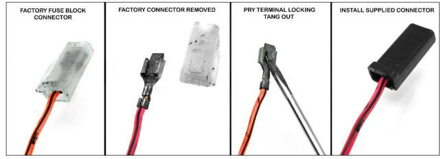
Install one of the single-pin connectors on each of the factory wires and connect them to the Painless harness. The factory pink/black wires connect to the power window, YELLOW #911 wire on the Painless harness. The factory, orange/black wire connects to the power lock, YELLOW/BLACK #910 wire on the Painless harness
