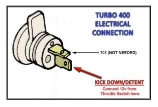
• If you have a factory, accelerator pedal mounted switch, you can use a switched power source inside the vehicle or you can route the cutoff piece of **#954** to the interior, connect at the throttle switch, and then route it back out to the transmission.
