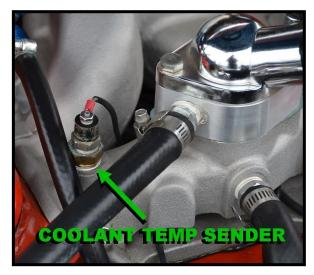
• Route this **GREEN #921** wire to the coolant temp sensor, cut to length, strip ½" insulation, and crimp on the appropriate terminal for your connection, and connect.
