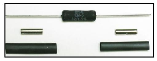
\*In factory applications where this alternator was used, a charge indicator light created the necessary resistance. For those with an instrument panel with a charge indicator light, the resistor is not needed. However, the #914 wire needs to be routed to one side of the charge indicator light and the other side of the light then routes out to the alternator. A charge indicator light was explained in more detail on page 50.
