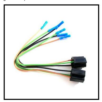
If your vehicle is equipped with dual/quad headlights, meaning the vehicle has a high/low beam light and also a separate high beam light on each side, as shown below, additional pigtails will need to be purchased (Painless #80300). The LT. GREEN wire from one of these pigtails will also splice to the LT. GREEN #908 wire. See the diagram on page 36 for a visual reference.
