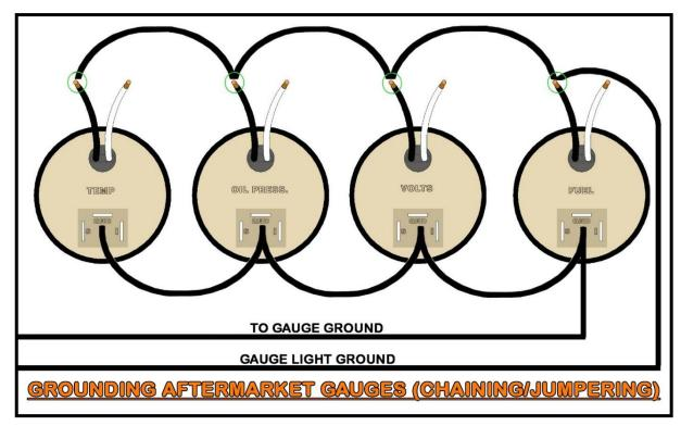
Gauge light power is supported by the **BROWN #930** wire. This wire connects to one of the leads for the gauge light or the gauge light tab found on gauges with LED backlighting. To make these connections you can splice from this **BROWN #930** wire to all the gauges or chain/jumper it all together.
