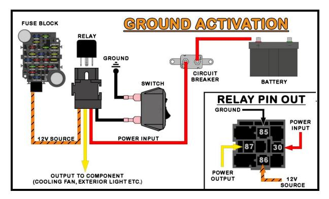
A ground activated relay is just the opposite of the 12-volt, activated relay; 12 volts (battery constant or switched) is supplied uninterrupted and the ground wire is switched. The Horn Relay pre-wired in the Painless harness is a Ground Activated Relay. Another example of this method is a thermostat operated fan relay. In this case, however, a thermostatic switch would replace the switch in the drawing above (see below).
