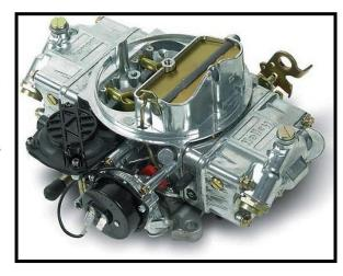
"choke thermostat." This spring will unravel as it is heated causing the choke to slowly open. When the ignition is turned to the "OFF" position, power is no longer on this wire, causing the spring to begin to cool and contract, closing the choke.
