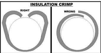
In the parts kit, you will see different uninsulated male and female terminals. These terminals are for factory-style connections and require rollover crimpers.
