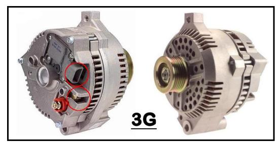
The two wires **RED** #995 **REGULATOR BATTERY POWER** and **WHITE** #914 **ALTERNATOR EXCITER**, connect to the pigtails on the back of the alternator.
