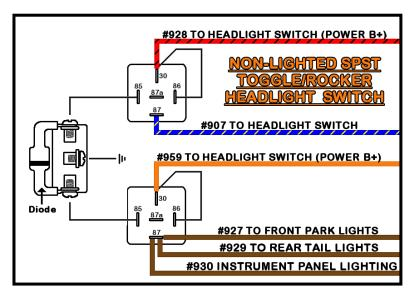
Those using a lighted toggle/rocker switch, connections are the same as a non-lighted only you will need to provide a power source to the backlight of the switch. This will generally be a tab on the back of the switch that is opposite of the terminals for the input and output(s) as seen below.
