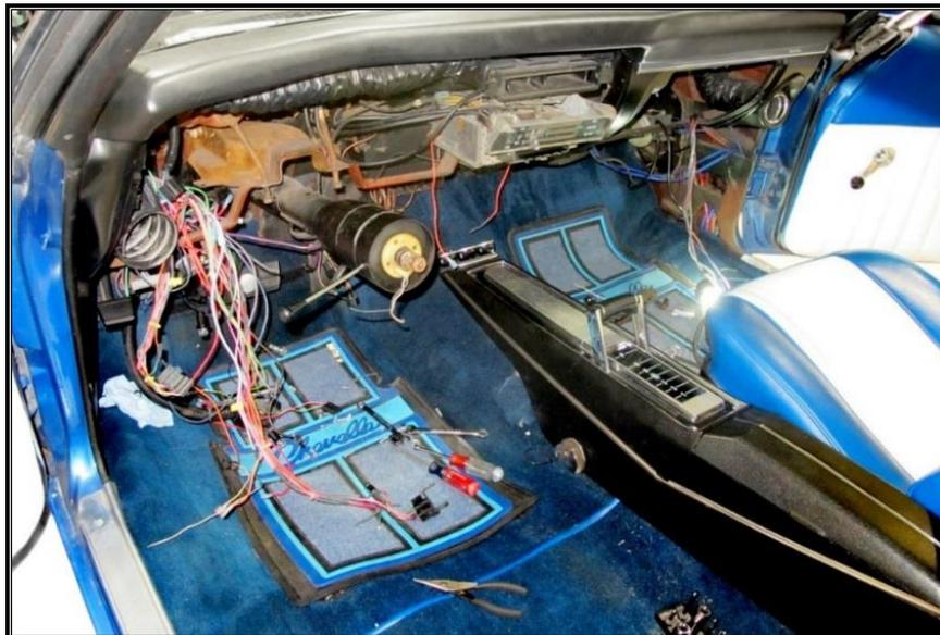
During the removal of the old, factory harness, avoid making any unnecessary cuts to any wires. The entire harness should be able to come out of the vehicle without any cutting at all unless someone has modified connections.
