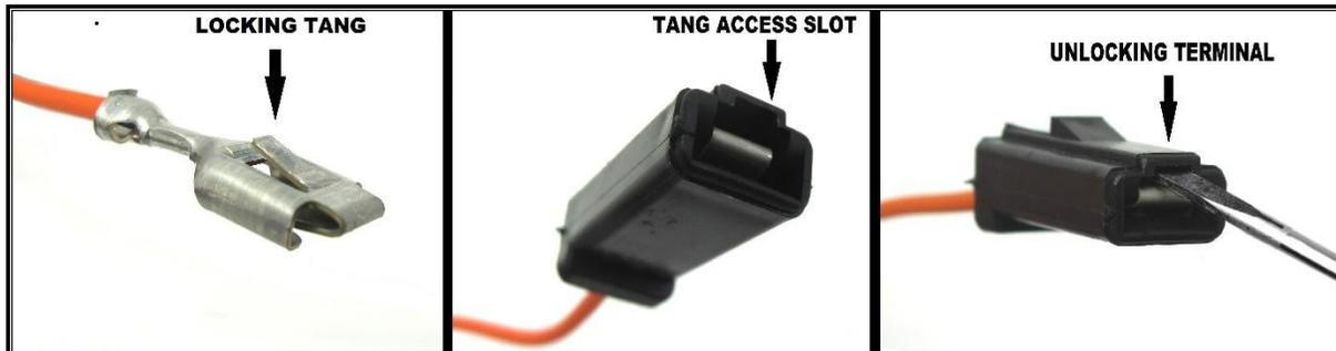
With this harness being universal, many of your factory connectors or factory service pigtails will need to be re-used. Factory terminals have been provided to allow re-using the connector without having to splice to existing wires. The removal process of wires into factory style connectors is as followed:
