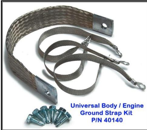
You have probably noticed the large cable coming from the negative side of your battery going down to the frame or the engine. This cable allows voltage to get back to the battery through the metal of the frame and all the other metal pieces bolted to the frame. It is also important to have ground cables going from the frame to the engine and from the frame to the body.
