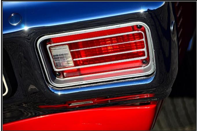
Separate turn brake signal vehicles will usually have 2 or 3 sockets: 1 socket with dual filaments (brighter filament for brake, dimmer for tail) and 1 socket with a single filament for the turn signal. Remember to count the bulb filaments or the contacts on the bottom of the bulb, not the wires going to them, as your sockets may or may not have ground wires.
