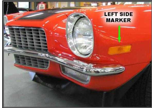
The park light feature is activated by a power source coming from the headlight switch. This light illuminates any time the headlight switch is in the “PARK” or “ON” position. The turn signal feature is provided by a power source coming from the turn signal switch.
