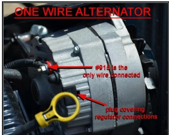
Locate the two wires intended for regulator connections; they will be grouped together in the **Engine Section**. These wires are:
