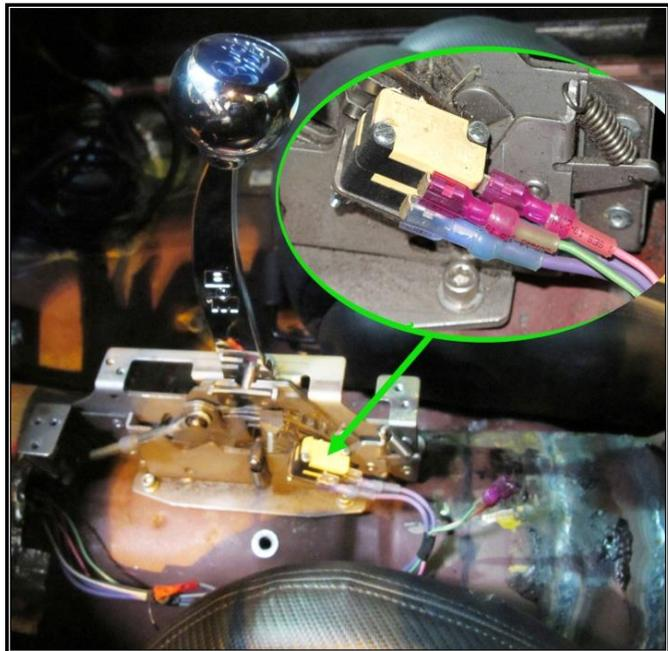
Small insulated terminals have been provided in the parts kit to accommodate aftermarket shifter switches.
