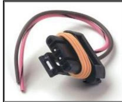
In factory applications where this alternator was used, a charge indicator light created the necessary resistance. **For those with an instrument panel with a charge indicator light, the resistor is not needed**. However, the **#914** wire needs to be routed to one side of the charge indicator light and the other side of the light then routes out to the alternator. A charge indicator light was explained in more detail on [page 53](#).
