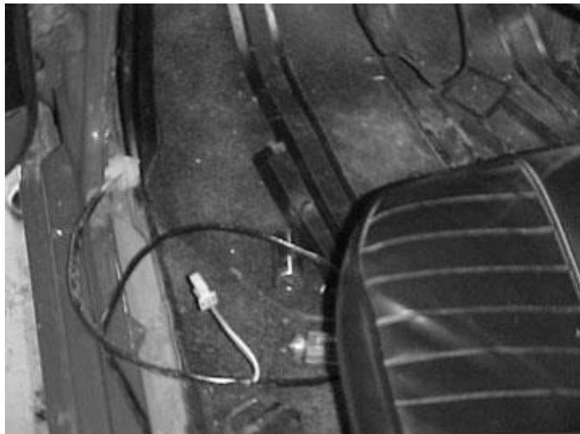
Figure 8.6 Driver Kick Panel and Jamb Routing
