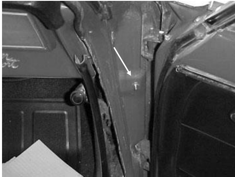
Figure 8.5 Door Jamb Switch
