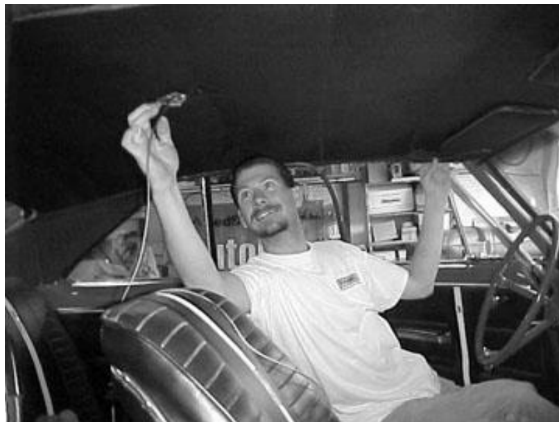
Figure 8.4 Routing Dome Light Wires
