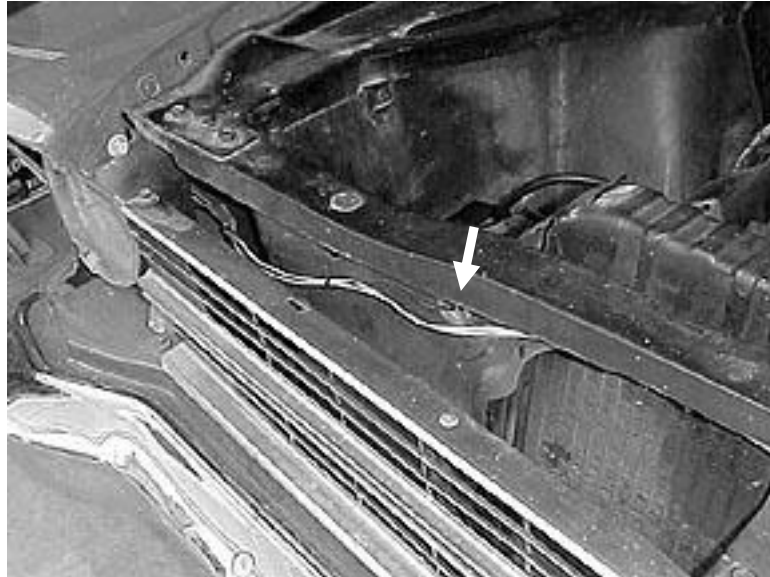
Figure 8.19 Passenger Side Headlight Wire Routing
