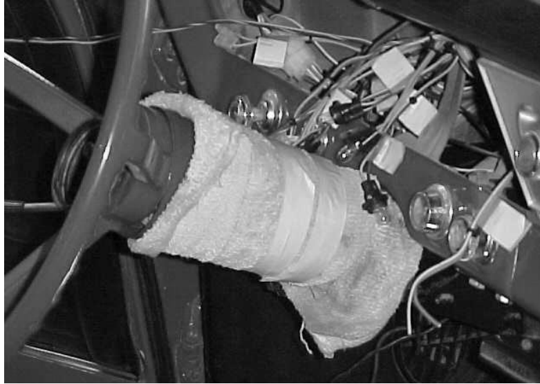
Figure 8.23 Steering Column Covered for Protection
