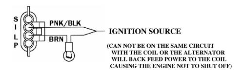
NOTE: WHEN NOT USING A CHARGE LIGHT A 82, OHM 5 WATT RESISTIOR (PROVIDED) MUST BE USED TO PREVENT PREMATURE FAILURE OF THE REGULATOR.
