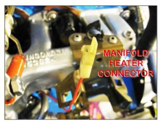
If you do not have roll over crimpers, heat shrinkable insulated push on terminals have been provided. These will allow for a good connection to the manifold heater connector, however, it will not be as attractive as the factory style terminal/connector connection the roll over crimpers will allow.
