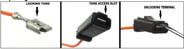
Notice the locking tang that holds the terminal in the connector. Locate the tang access slot on the terminal end of the connector. The connector in the photo is just an example and not a connector found on the 30814 harness. Push a paper clip, stiff wire, or a small flat head screwdriver into the slot to depress the locking tang on the terminal.
