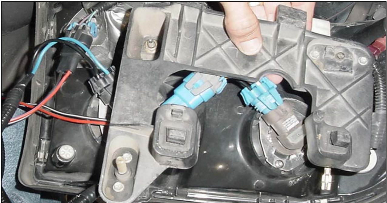
Illustration 3 Painless Headlight Relay Harness plugged into headlights
