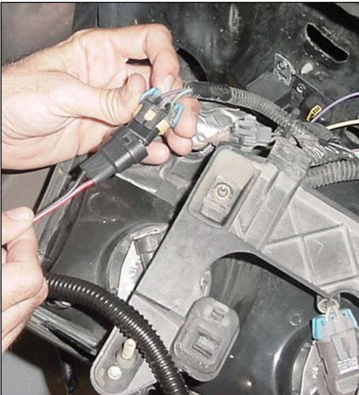
Illustration 2 Connection of the Painless Headlight Relay Harness to vehicles factory harness
